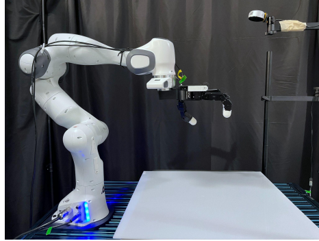
Figure 15: Our physical experiment setup including a Frank Panda robot with an attached Allegro Hand. The camera is only used for high-level path planning.
